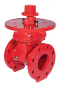
Flanged non rising stem resilient seated gate valve equipped with indicator post flange (post BX5900 is not included) for fire protection and fighting applications.
