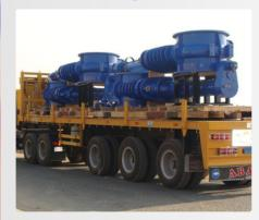
stem metal seated gate valves DN900 and DN1200 to Al Ameriya Sewage Lift Station, located in the heart of Cairo, Egypt. These valves had a 30 meter long extension spindle and were electrically operated. The successful supply and installation of these valve marked a milestone in BIMEX history of success.
